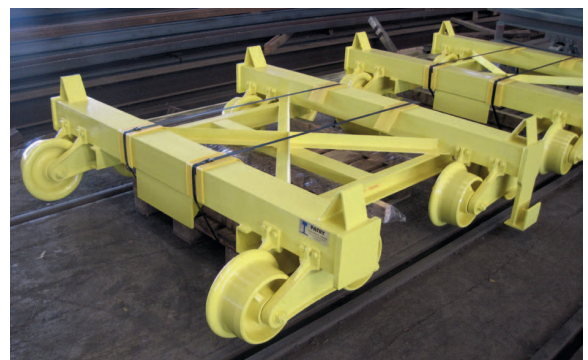
Chariot manuel 4 T Manual trolley, load 4 T
