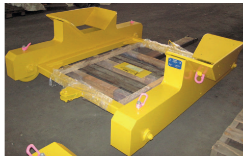
Chariot manuel 8 T Manual trolley, load 8 T
