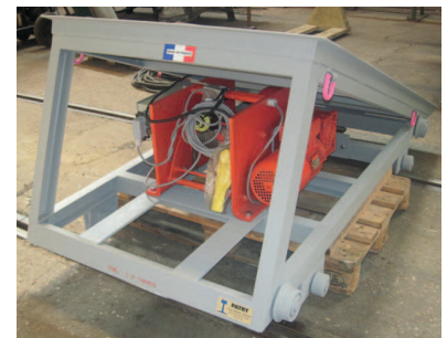
Chariot manuel 1 T Manual trolley, load 1 T
