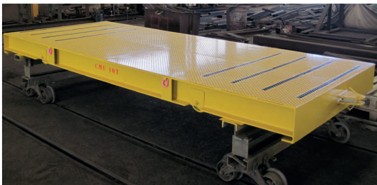
Chariot manuel 18 T Manual trolley, load 18 T
