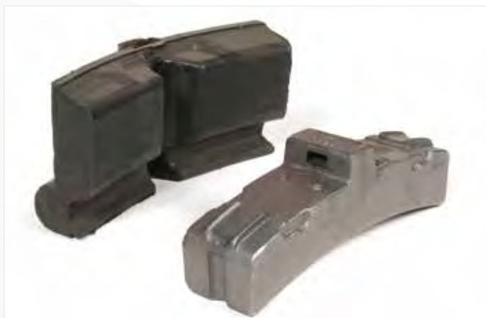
Semelles de frein fonte ou composite Brake shoe made of cast iron or composite
