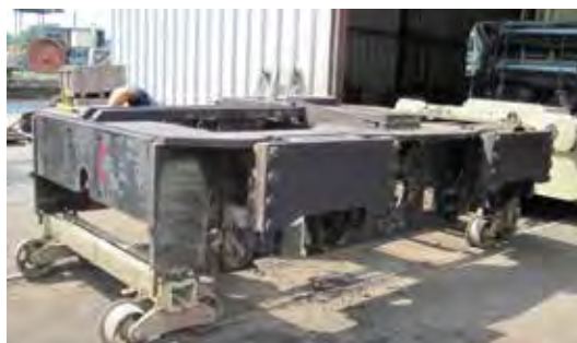
Chassis boggie de locotracteur BB Fauvet Girel 72 t Chassis of a boggie from locomotive BB Fauvet Girel 72 tons
