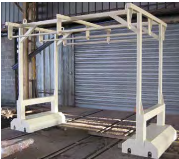
Lorry suspente 1 T, cabine pour peinture Specific lorry 1 T, for painting booth
