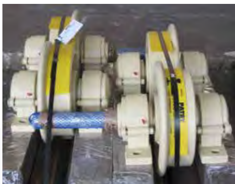
Roues entre paliers 97-3 motorisable 400 M Wheels 400 M between bearers with 97-3 assembly (axle adjustable to engine )
