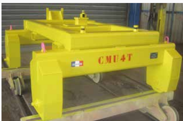
Chariot manuel 4 T, support moteur Manual trolley load 4 T for engine handling
